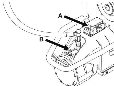
Once the power cable is connected to the saw, the carabiner on the cable must be attached to the saw unit to prevent pressure on the plug when in operation. The carabiner must be fastened to one of the bracket eyes on the handle which is screwed to the back of the drive motor.
