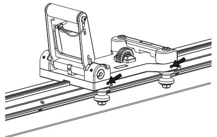
Press down the locking device and pull the saw carriage in both directions by hand. Carriage should slide easily with a slight resistance. All 4 guide wheel should spin.
