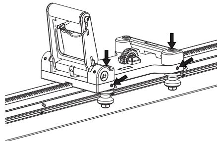
Turn the shafts gently with a 16mm wrench until the guide wheels rest agains the rail.
