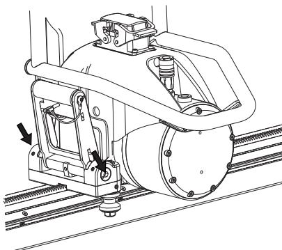
Tighten the two stop screws with a 3 mm allen key.
