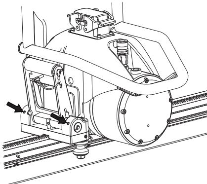
Turn the two excenter sleeves with a 8 mm allen key until the shaft is tight and parallel to the saw unit.
