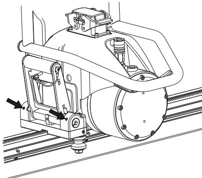
Make sure the locking handle is properly adjusted by open and close and see that the spring loaded lock is in locked position.
