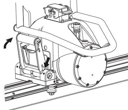
Then secure the locked handle with the locking pin.
