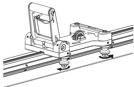
Hold the 16 mm wrench in position and tighten the two stop screws with a 3 mm allen key.
