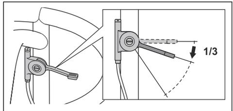
3. Set the choke control in the correct position.
