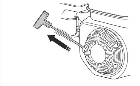
6. Release the starter rope handle to let the starter rope go back.
