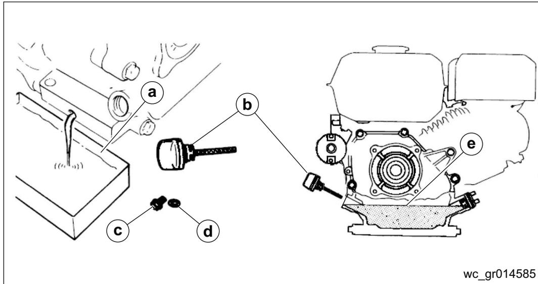
2. Remove the filler cap/dipstick (b), drain plug (c), and washer (d).
