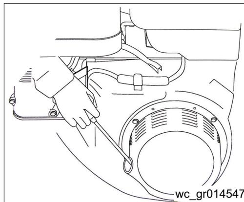
**NOTICE:** Do not allow the starter grip to snap back against the engine. Return it gently to prevent damage to the starter.
