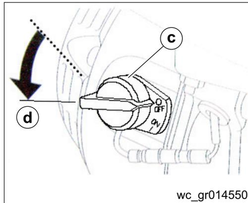
3. Turn the fuel valve lever (e) to the OFF position (f).
