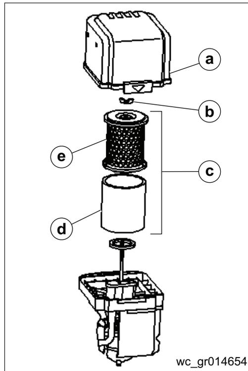
2. Remove the wing nut (b) from the air filter assembly (c) and remove the assembly.
