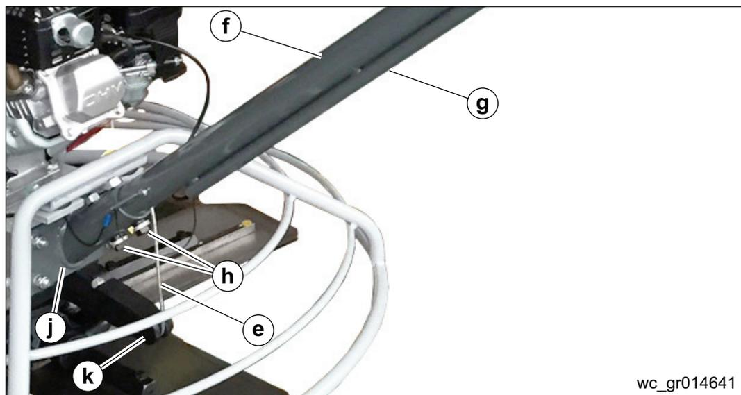
2. Remove the two bolts (h) and two nuts from the bottom end of the handle.
