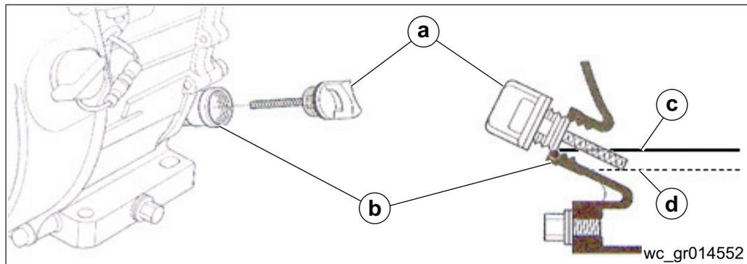
2. Insert and remove the dipstick without screwing it into the filler neck (b).
