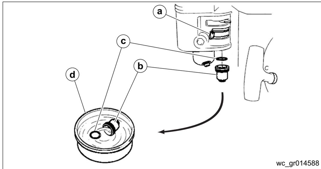
2. Remove the sediment cup **(b)** and O-ring **(c)** and place them in a suitable container **(d)**.
