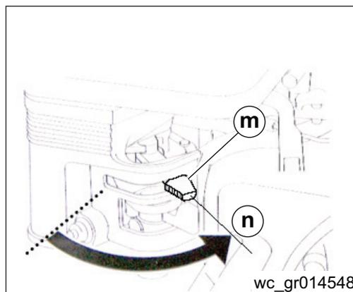
7. Adjust the throttle lever the desired position to set the engine speed.
