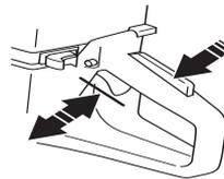
Start the machine, release the switch, and check that the machine and blade stop.
