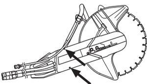
Take off the old belt and fit the new one. Fit the cutting arm to the machine and tension the belt with the adjuster screw. A new drive belt should be re-tensioned after running for about 30 minutes.
