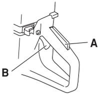
The switch lock remains pressed as long as the switch is pressed. When you release your grip on the handle this resets both the switch and the switch lock. This takes place via two independent return spring systems. This position causes the machine to stop and the switch to be locked.
