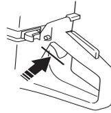
Press the switch lock and check that it returns to its home position when released.
