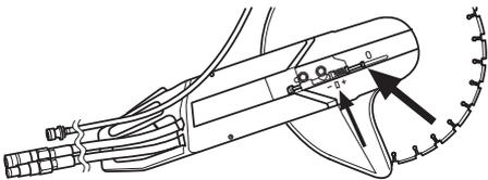
Tighten the two nuts holding the cutting arm.
